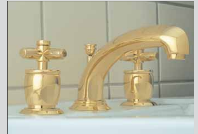
MB1929XMIB Deck mounted Zephyr spout lavatory faucet in Inca Brass with cross handles. 4 7/16" high fixed spout with 5 1/2" reach
